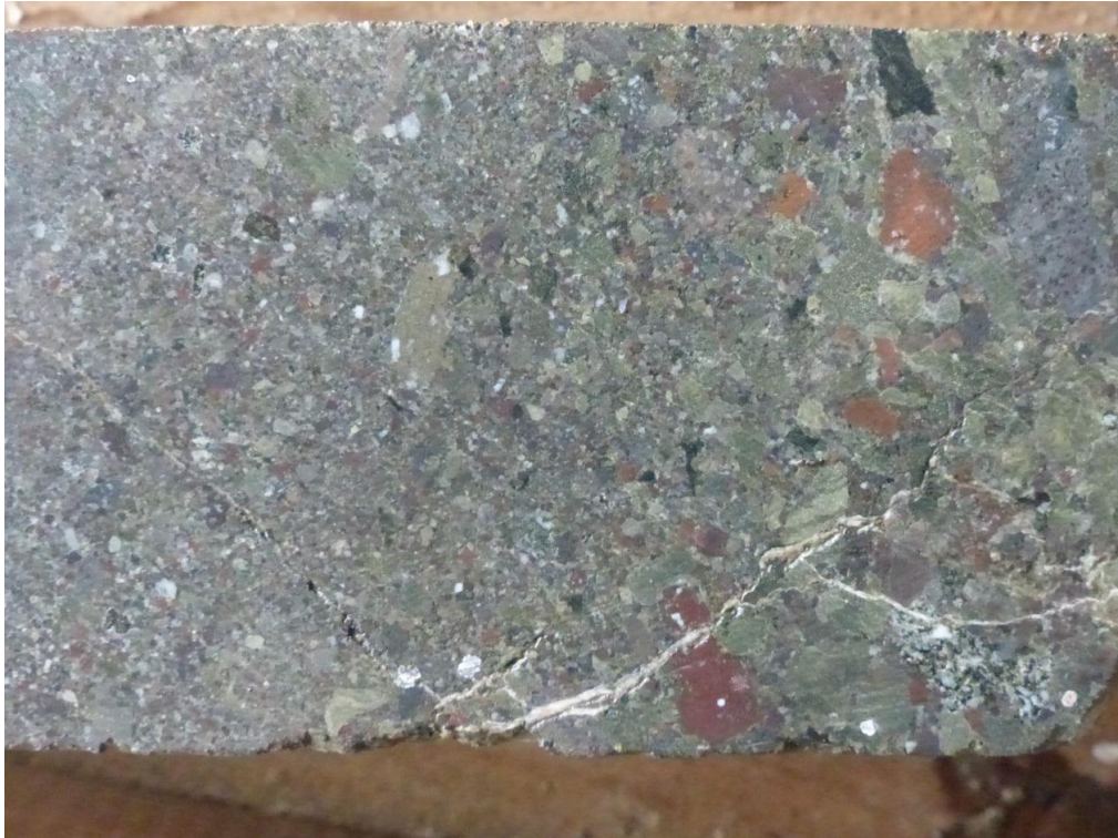
36. Polymictic Volcaniclastic Breccia with fragments of andesite and dacite in an heterogeneous groundmass showing only crude banding. DDH 10-64m.
