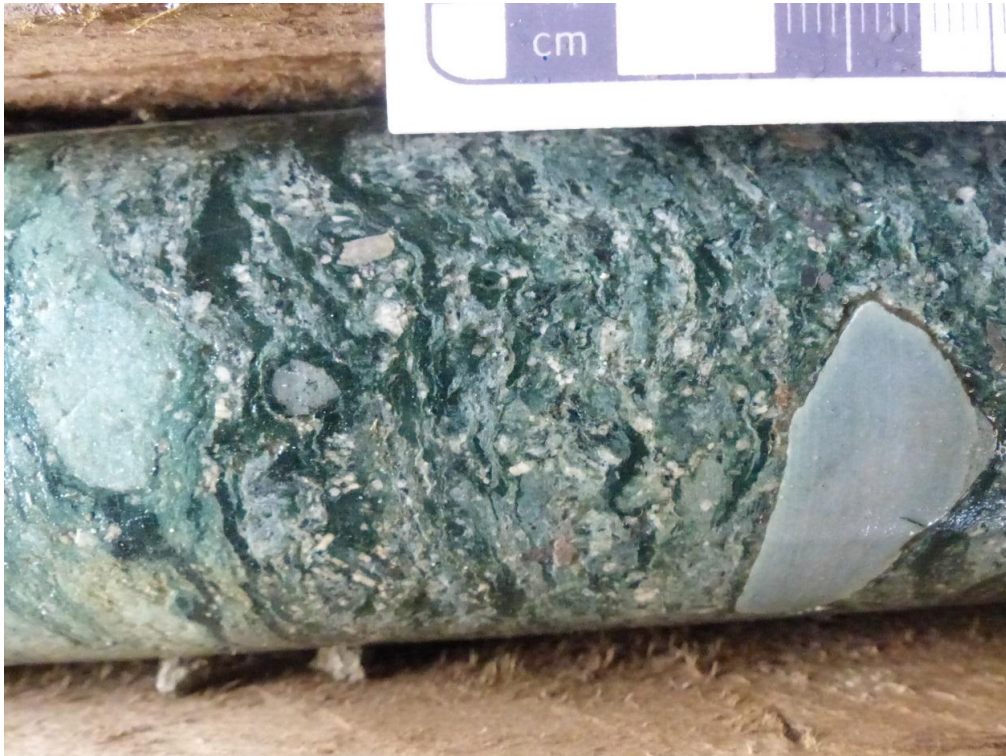
46. Breccia interbedded in the Crystal - rich Polymictic Breccia with cm - sized fragments of aphyric rhyolite and likely related to the late rhyolite domes. This rock is similar to that described as the “grainstone” in the deposit. DDH 11-106m.
