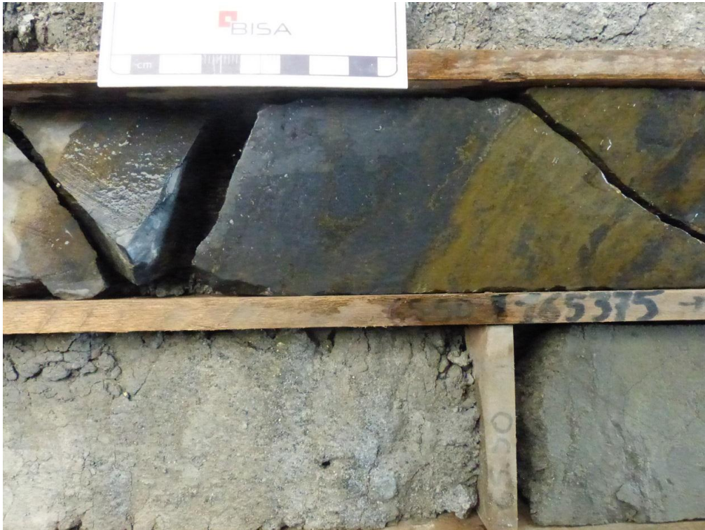
34. Upper contact of the massive sulphides with the Polymictic Volcaniclastic Breccia via a 40 cm thick band of fine grained grey silica. DDH 11-106, 78 m.
