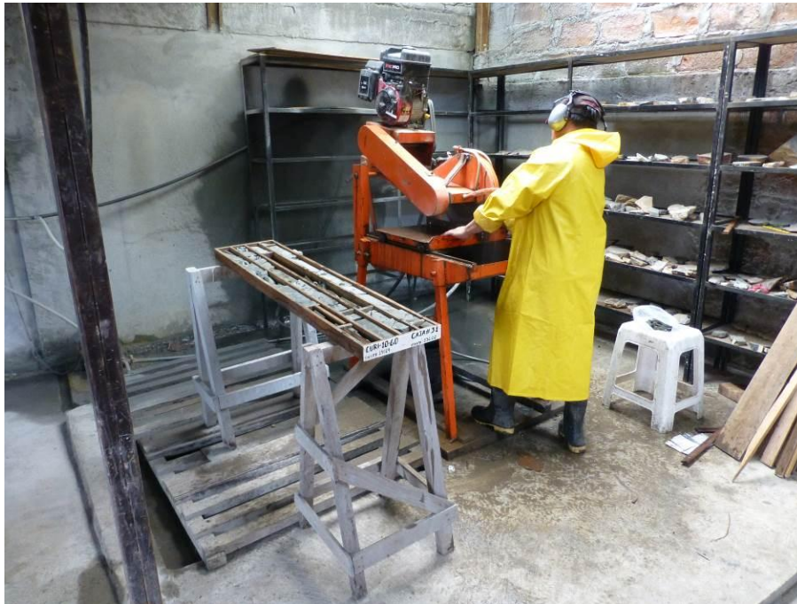
FIGURE 11.2 SAMPLE CUTTING WITH A DIAMOND SAW
