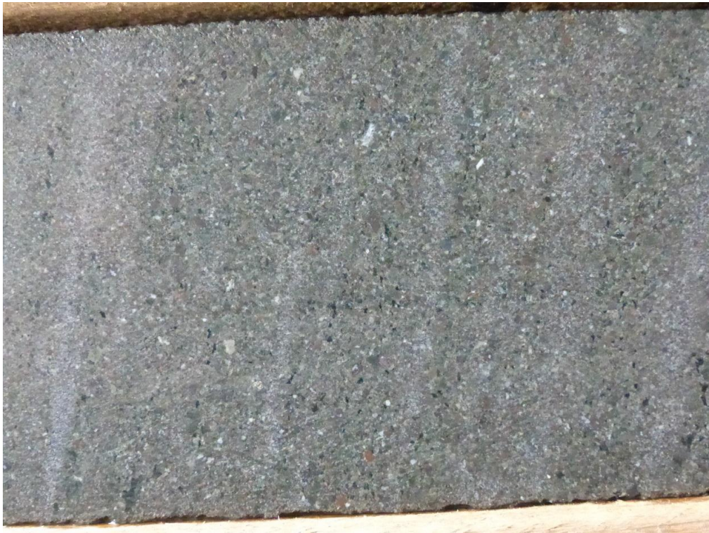
37. Fine - grained polymictic volcaniclastic breccia with local grading and crude banding. DDH 10-64m.
