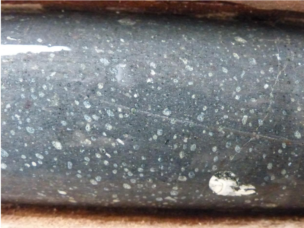
42. Vesicular basalt that delineates the upper part of the subvolcanic sill. DDH 10-68m.
