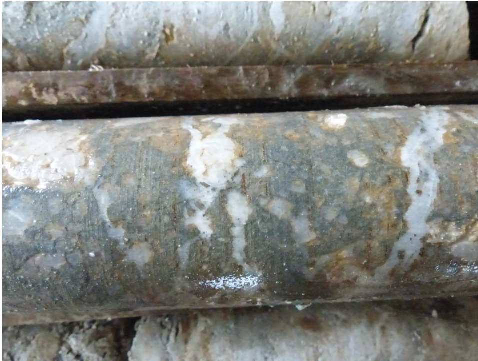
11. Rhyodacite pervasively replaced by a quartz-sericite-pyrite-(chlorite) alteration and crosscut by anhydrite-rich veins. DDH 10-64 m.
